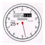
The 0 on the far right is a fixed number and never changes. Each number on the round dial represents one gallon so from 0 to 1 is one gallon, 1 to 2 is one gallon, etc. One complete turn of the read needle is 10 gallons.
